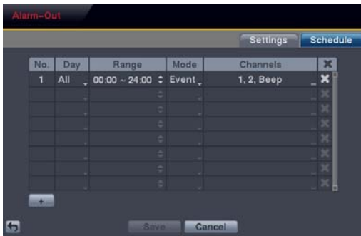
Figure 29 — Alarm-Out Schedule screen.
