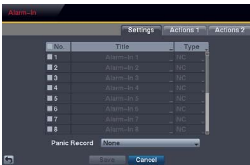
Figure 42 — Alarm-In Settings screen.
