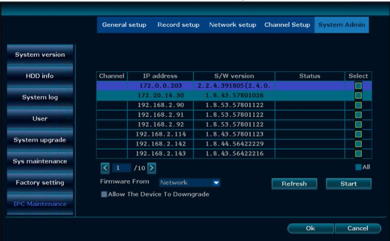
2, Put the prepared IPC firmware into the USB flash disk, insert it in to the USB Port behind the recorder. Check the
