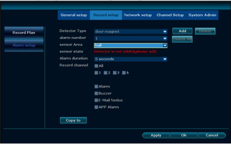
3, Select the alarm type, alarm serial number and alarm area, trigger the type of alarm, click "Add". Waiting 30 seconds, there will prompt "add success".
