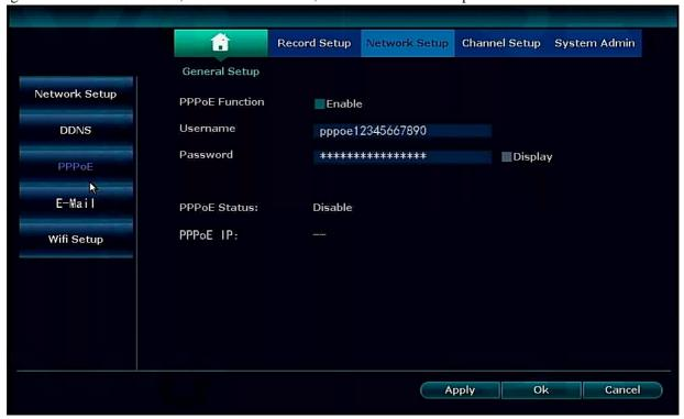
2, Check the Enable box, in the edit box, enter the user name and password provided by ISP.
