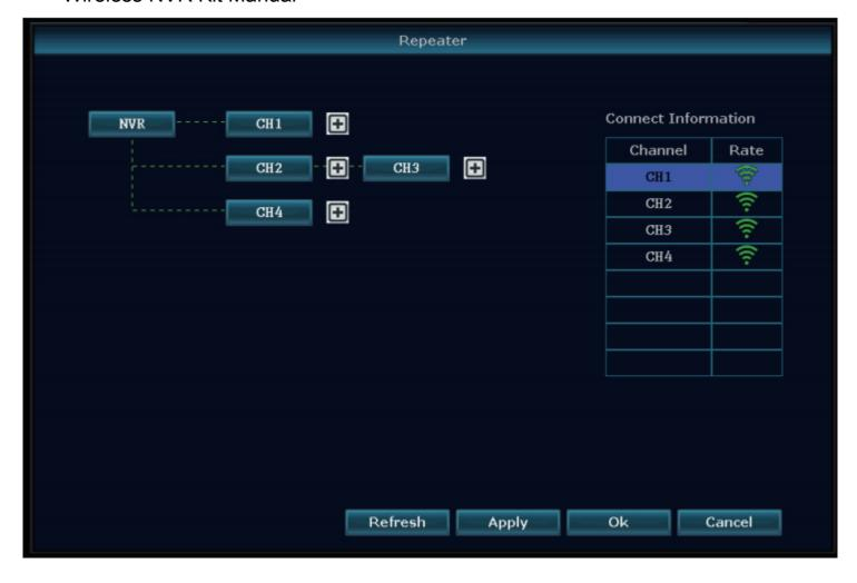
3, As the picture shows below, IPC3 is connected to the NVR through IPC2 and IPC1. IPC2 is connected to the NVR through IPC1. IPC1 and IPC4 are connected to the NVR directly.
