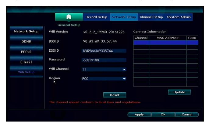
Click Reset to restore the information of the wireless module to the factory setup.
