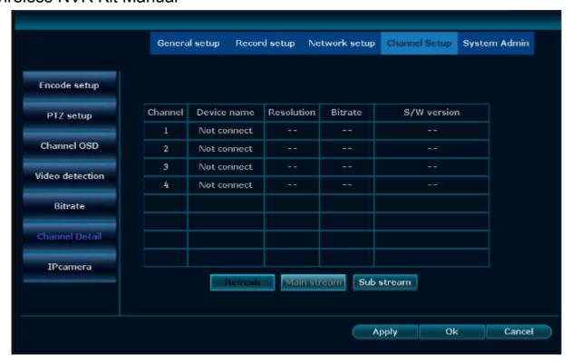
2. Click Refresh, you can search the camera in current channel and you can check the channel name of the device, resolution, stream value, video frame rate, software version details.
