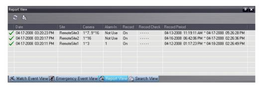
The Report View panel displays the system status information of remote sites. REVO Remote Pro checks the remote site and reports system status. Clicking the configured during REVO Remote Pro System setup for this feature to function. Refer to 3.3 Menu – System Menu for more details.
