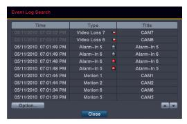
The DVR maintains a log of each time the Alarm Input port is activated. The Event Log Search screen displays this list. Use the arrow buttons to highlight the event for which you would like to see video.
