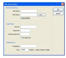
Remote Site Setup: Enter the site name and IP address of the DVR connected to the devices you want to include on the map. Click the Port... button and enter the network IP port number (8000 to 12000) that matches the value set during the LAN setup on the DVR. Check the box beside Use DVRNS to use the DVR name service.
