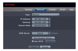
Type: Select the type of network configuration from: Manual, DHCP and ADSL (with PPPoE).
