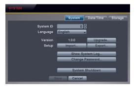
System ID: Set the system ID. Use the Up and Down arrow buttons or scroll the mouse wheel to increase or decrease the number.
