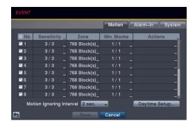
No.: Your DVR has built-in motion detection. Selecting the box turns the motion detection On and Off for each camera.
