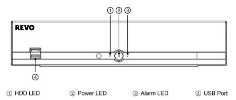
NOTE: The infrared sensor on the DVR is just to the left of the HDD LED. Make certain that nothing blocks the sensor, or the remote control will not function properly.
