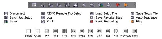
Select the desired screen layout using the layout toolbar. When changing the screen layout, the selected camera on the current screen will be located in the first cell of the new layout. When in one of the multi-view formats, clicking the or button will move to the previous or next page.
