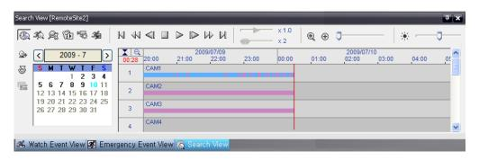
The Search View panel allows time-lapse or event searching of recoded data on the remote DVR.
