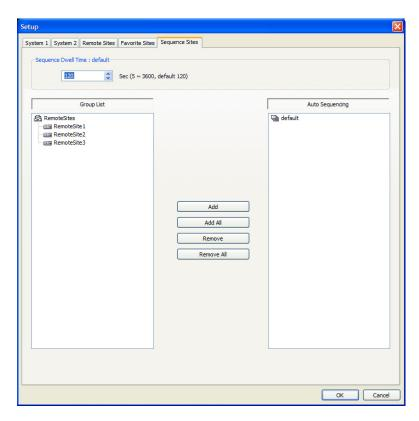
**Sequence Site:** Configure the sequence site. REVO Remote Pro connects to the registered sites sequentially allowing connection to more than one remote site. Register an Auto Sequencing group and add desired sites in the Group List to the Auto Sequencing group. Video from the sites added to the Auto Sequencing group is displayed on the screen in the preset sequence interval during the sequence monitoring.
