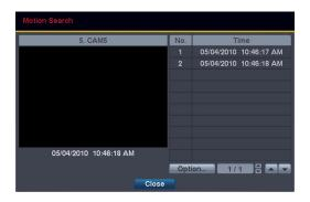
Motion Search can be selected from the Search menu while the DVR displays the camera full screen. The Motion Search screen displays a list of motion events. Use the arrow buttons to highlight the event for which you would like to see video and press the 🔁 button to display the video associated with the selected event in the small search screen.
