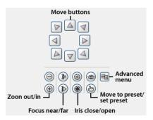
Select a PTZ camera at the remote site, and control pan, tilt and zoom. Only the administrator can control PTZ at REVO Remote Pro. The Picon will display on each camera screen when PTZ can be controlled remotely.
