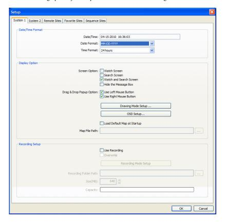
System 1: Set up the date/time format for REVO Remote Pro, display option, and panic recording function.
