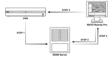
STEP 1 (DVR → DVRNS Server): Register the unit name and IP address of the DVR during the DVRNS setup on the Remote DVR. This unit name and IP address will be registered on the DVRNS server directly.
