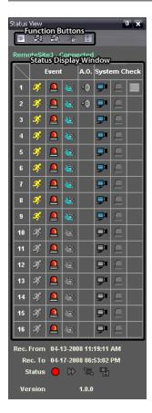
REVO Remote Pro provides a status display, remote setup, system log and event log view of the connected remote site in real-time. To display the status of the remote site, select a camera or a site from the Remote Site list and drag it to the Status View panel. You can also select Connect Status from the popup menu displayed by clicking the right mouse button after selecting the site from the Remote Site list.
