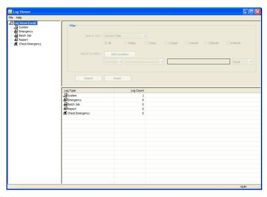
**View Log:** Displays the type of log and the number of log entries of REVO Remote Pro. Selecting a log type from the list displays all entries of the selected log type, and you can search for the desired log by setting up a search filter.
