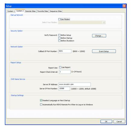
**System 2:** Set up the modem connection information for remote access, system password, network option, report function, and DVRNS server.
