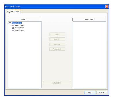
**Setup:** Sets up the remote setup job for remote sites. First, select the remote sites to set up from the Group List, and add them to the Setup Sites list by clicking the Add button. Then, click the Setup Now button to initiate the remote setup job for Setup Sites.
