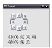
The panel allows PTZ control while live monitoring a remote site.
