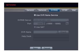
NOTE: The DVRNS (DVR Name Service) allows you to connect to the DVR, via internet, with the dynamic IP address or the domain name. To make this feature easy, you can name your DVR (example: TomStore05) and connect using the DVR name instead of the IP address. To use the DVRNS feature, you will need to have your DVR registered through DVRNS with the settings matched between your DVR and the DVRNS server. Any changes to the DVRNS server might cause improper operation.
