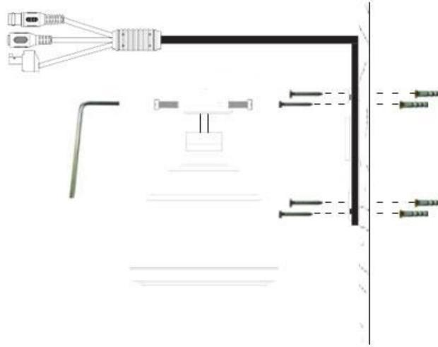
Connect the camera's BNC video cable and RS-485 wiring to your DVR and (optional) joystick keyboard.
