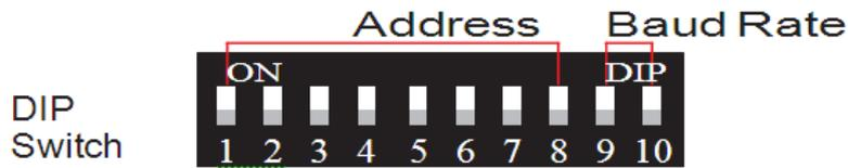
Set DIP switches 1 (least significant bit) through 8 (most significant bit) to set the RS-485 address of the camera. The address can be set from 0 through 255, and must be matched to the RS-485 address (often called the “ID”) in use by the controlling DVR or joystick keyboard. Once set, the camera’s address does not need to be changed. If more than one RS-485 device is connected using the same RS-485 wiring, make sure that each device has a different address.
