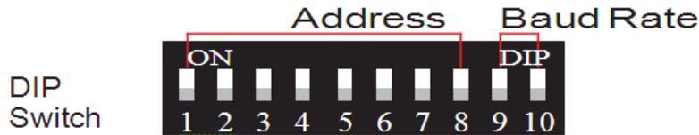
Set DIP switches 9 and 10 to set the RS-485 baud rate of the camera. The baud rate can be set to 2400, 4800, 9600, or 19200 bps. Make sure that the baud rate of the camera matches the baud rate of the controlling DVR or joystick keyboard.
