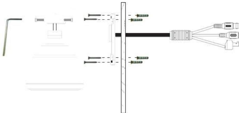
Drill holes in the mounting surface, and affix the camera using the supplied screws and plastic anchors. The BNC video cable can go straight through an additional, larger hole drilled into the mounting surface, or against the mounting surface using the slot at the bottom of the camera's base.
