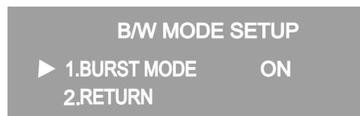
◆ **AUTO** : The mode is switched to 'Color' in a normal environment, but switches to 'B/W' mode when ambient illumination is low. To set up the switching time for AUTO mode, press the Function Setup switch. You can turn on or off the burst signal on B/W mode.
