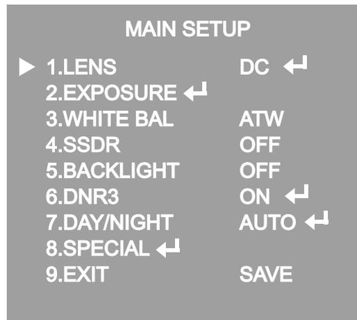
2. Select a desired function using the Function Setup switch.
