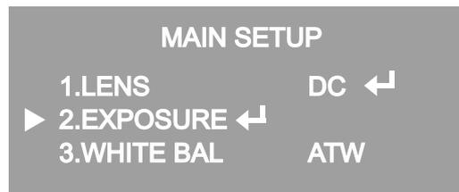
1. When the SETUP menu screen is displayed, select 'EXPOSURE' by using the Function Setup Switch.
