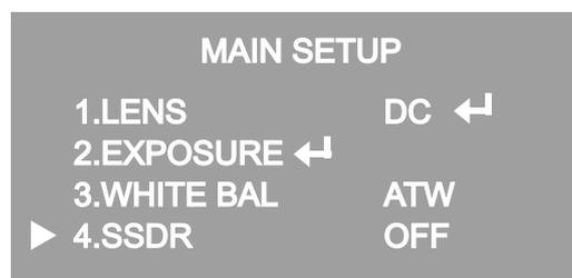
1. When the SETUP menu screen is displayed, select 'SSDR' by using the switch so that the arrow indicates 'SSDR'.
